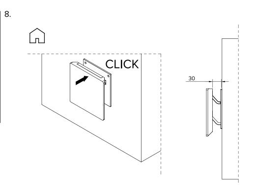
Connect the elements by snapping the upper part into the body
