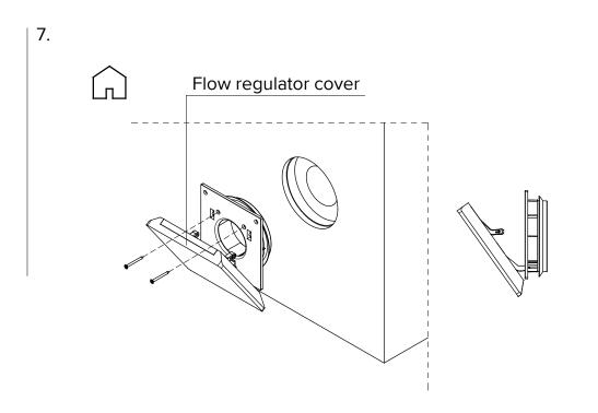
After plastering the wall and finishing the interiors, insert the flow regulator into the pass-through duct until it stops. Lower the flow regulator cover in order to expose the screw holes. Screw the flow regulator into the wall with screws
