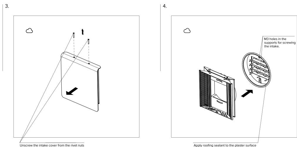
using two screws, using hexagonal key 2mm
