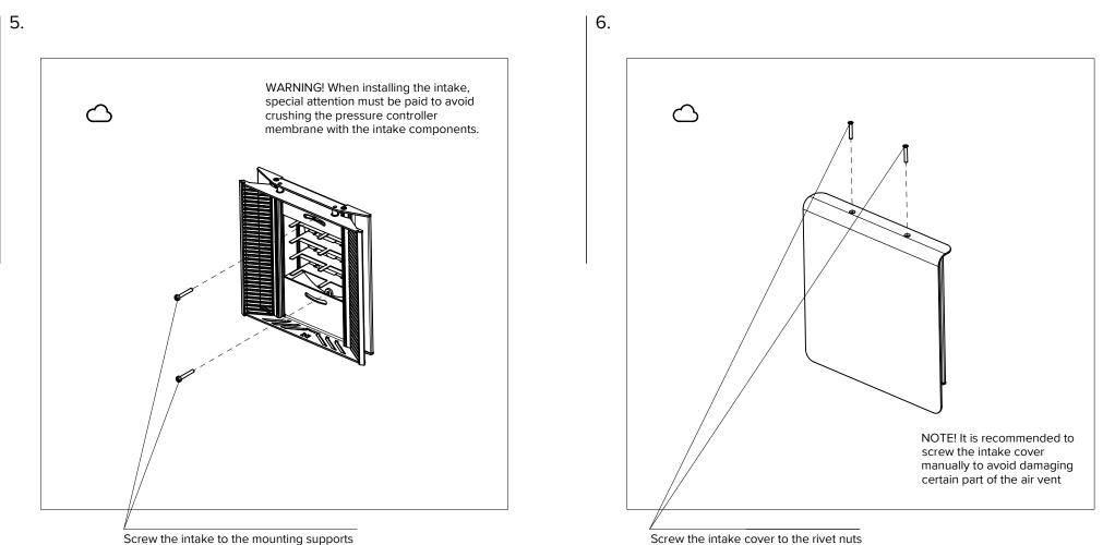
Screw the intake cover to the rivet nuts using two screws, using hexagonal key 2mm
