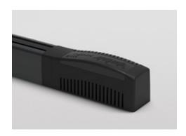
The controller mechanism is based on a small, precise device which measures relative humidity in the room and directly adjusts the air flow while adapting the ventilation performance to the humidity level.
